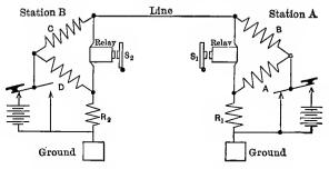
FIG. 174. Bridge Duplex Telegraph Circuits.
